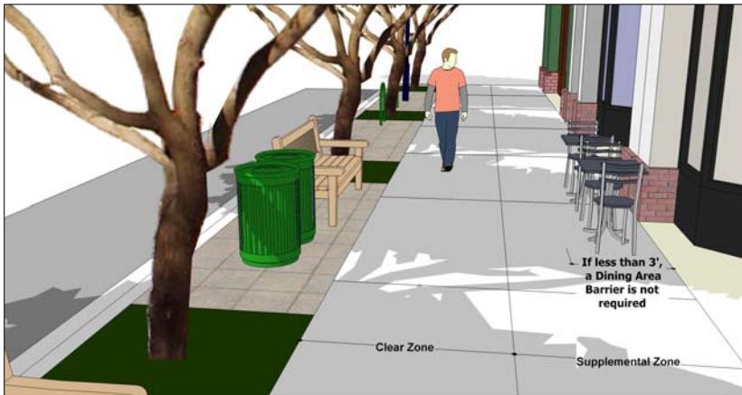
Sidewalk Dining: No dining barrier required:
